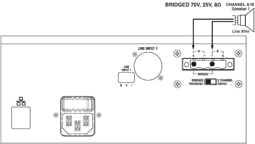
**Figure 1. Bridged Wiring Diagram**
