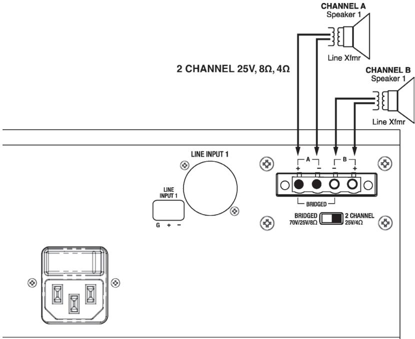
**Figure 2. Two-Channel Wiring**
